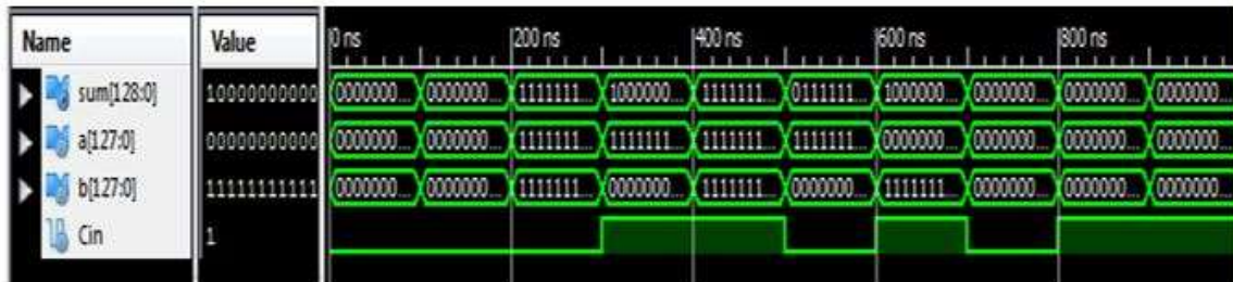
Fig 13: Simulation results obtained for the 128 novel bit adder
